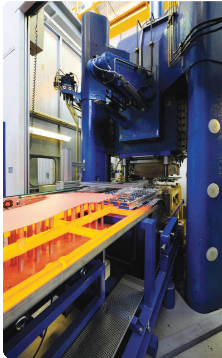
FIGURE 1. Hot stamping press in the test facility of ThyssenKrupp Steel Europe AG.
