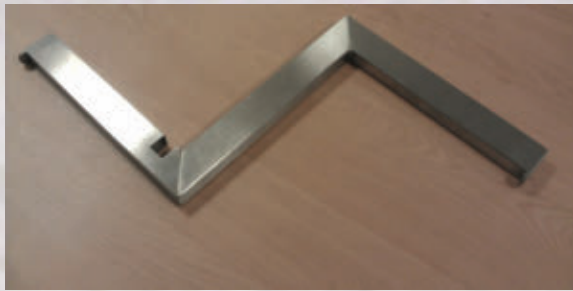
FIGURE 4. A demonstrator component welded with disk laser technology.
